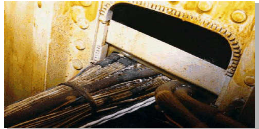
DRILL SHAVING AND CONTAMINATION ON WIRE BUNDLES
